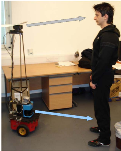
Fig. 1. Pioneer robot with laser and camera for legs and face detection.
