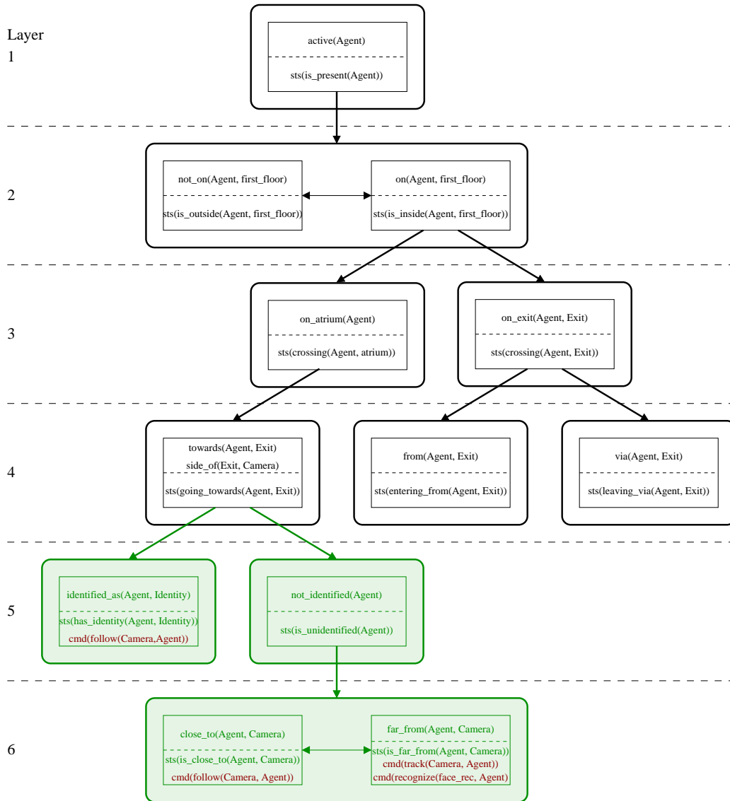
Figure 8: SGT for active camera selection and face recognition.
